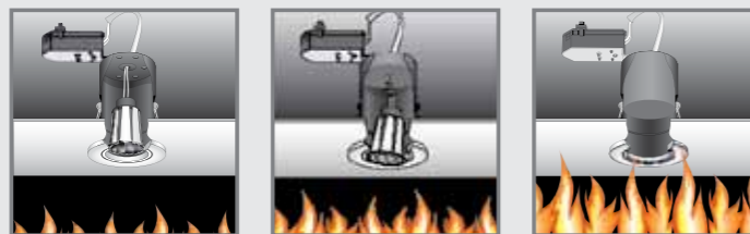
Fire starts Intumescent material expands Material seals the fire barrier
