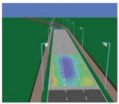
Scheme: Traffic route, 3 lanes, opposite arrangement. Total width 10.95m Luminaire(5) used: Triumph 1 150W HST, 10m mounting height, 36m spacing, 5° tilt Roadt  $L_{\alpha} = 5.75$  cd/m<sup>2</sup>;  $E_{\alpha\nu}/E_{\alpha} = 0.59$ ; Threshold increment = 2%
