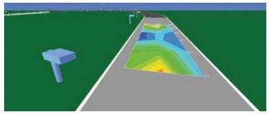
Scheme: Access ramp, width 4m Luminaire(s) used: Orus 70W CDM-T, 0.9m mounting height, 10.5m spacing Road:  $E_{\rm ov}=33~{\rm lux}$ ;  $E_{\rm min}=15~{\rm lux}$
