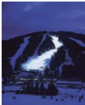
A ski slope lit using 270 Mundial 2kW floodlights. The floodlights are positioned and aimed to prevent glare to skiers, whilst revealing the texture of the surface of the slope to ensure safety. This requires aiming away from the direction of view of skiers, and the use of glancing angles to show surface texture. Additional care should be taken to prevent reflected glare from the snow.
