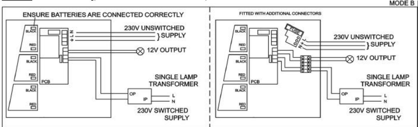
This unit is designed to be used with an external transformer (not supplied) which is used to power the downlighter as a normal lamp. This transformer may be separate from the downlighter fitting, or enclosed within it, in which case it is usually possible to cut the wiring from the output to the lamp and extend them to the unit.
