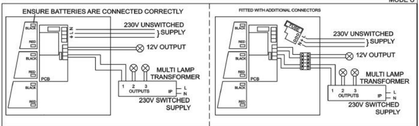
In this mode the transformer is rated large enough to power more than one lamp, (see manufacturers details for individual output terminals). One of these will be used as an emergency lamp. When the switched supply is ON all lamps will light, but only the EL lamp will light when there is a mains failure.
