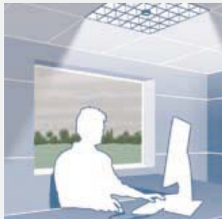
You are present. Insufficient daylight. Lights on.
