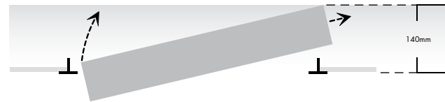
Fitting passed over one 'T' bar with one cross-noggin removed.
