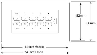
The module's enclosure and its supporting frame are designed to attach to the front of any standard Two-Gang Box, sinking, dry-lining or surface mounting, with a minimum depth of 30mm.
